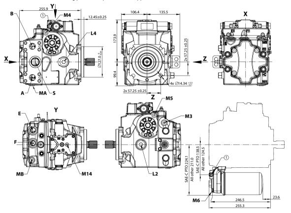
**A/B** system ports: Ø25.4–450 bar; Split flange boss per ISO 6162 **MA/MB** (system), **M3**, **M6** (charge) gauge ports per ISO 11926-1:  $\frac{9}{16}$ –18 **M4**, **M5** (servo), **M14** (case) gauge ports per ISO 11926-1:  $\frac{7}{16}$ –20 **L2**, **L4** – Case drain ports per ISO 11926-1:  $\frac{1}{16}$ –12
