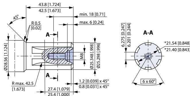
Straight-sided, bottom fitting, dep. Fit 2, Nom. size 1 in; \* Deviates from B.S. 2059 (SAE 6B)
