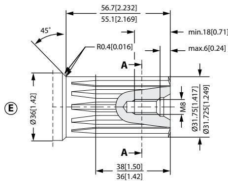
**E:** Involute splined shaft, ANS B92.1 - 1996 standard, Flat root side fit, Pitch 12/24, Teeth 14, Major dia. 1.25 inch, Pressure angle 30°
