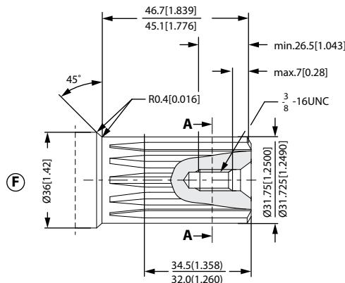
**F:** Involute splined shaft, ANS B92.1 - 1996 standard, Flat root side fit, Pitch 12/24, Teeth 14, Major dia. 1.25 inch, Pressure angle 30°
