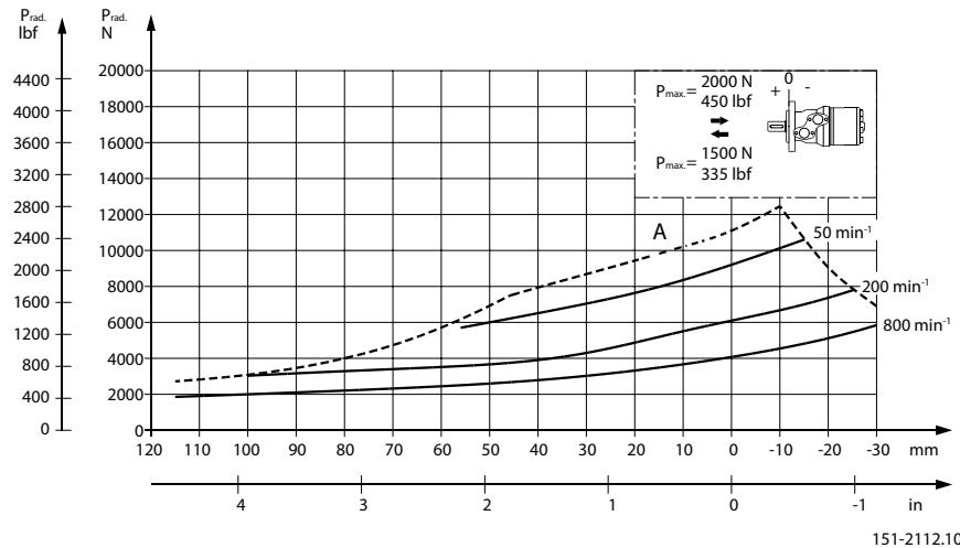
The output shaft on OMP N can be offered in needle bearings. These bearings and the recessed mounting flange allow a higher permissible radial load in comparison to OMP motors.
