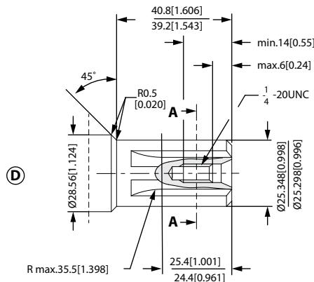
**D:** Splined shaft, SAE 6 B (B.S. 2059), Straight-sided, bottom fitting, deep. Fit 2, Nom. size 1 in
