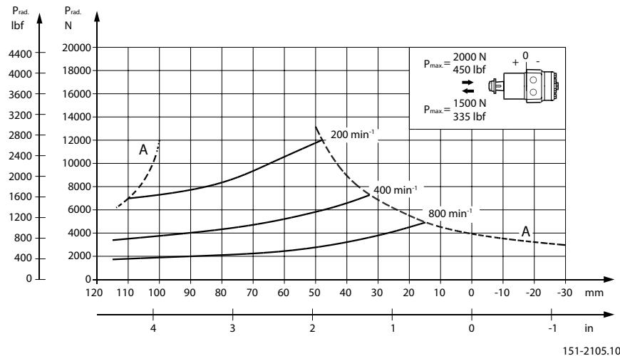
The output shaft on OMPW can be offered in slide bearings similar to the other OMP motors. The permissible higher radial load is therefore due to the recessed mounting flange moving the point of load closer to the motor bearings.
