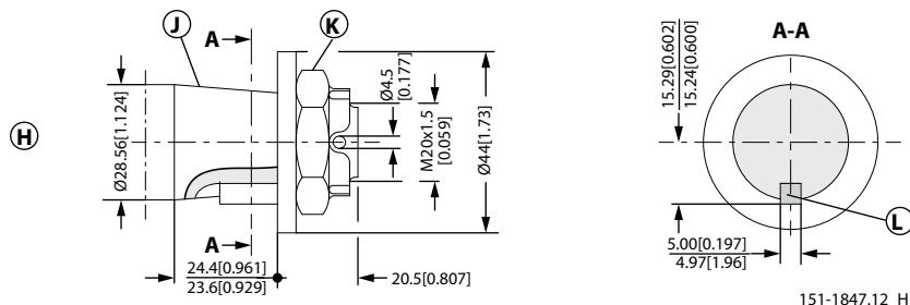
**K:** DIN 937 NV 30 Tightening torque:  $100 \pm 10 \text{ N}\cdot\text{m}$  [885 ± 85 lb·in]
