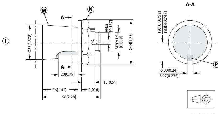
**N:** DIN 937 NV 41 Tightening torque:  $200 \pm 10 \text{ N}\cdot\text{m}$  [1770 ± 85 lb·in]
