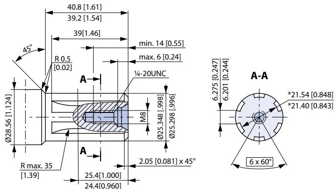
Straight-sided, bottom fitting, deep. Fit 2; Nom. size 1 in, \*Deviates from B.S. 2059 (SAE 6B)
