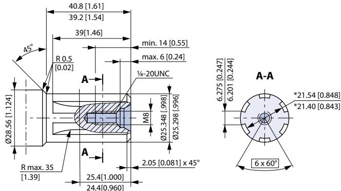
Straight-sided, bottom fitting, deep. Fit 2; Nom. size 1 in, \*Deviates from B.S. 2059 (SAE 6B)
