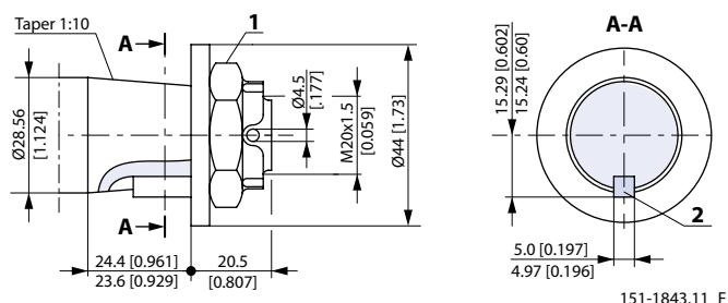
**1.** DIN 937 NV 30; Tightening torque:  $100 \pm 10 \text{ N}\cdot\text{m}$  [885 ± 88.5 lb·in]
