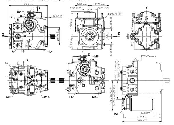
A/B system ports: Ø25.4 – 450 bar, Split flange boss ISO 6162; M1 2x 1.75, 20 min full thread depth
