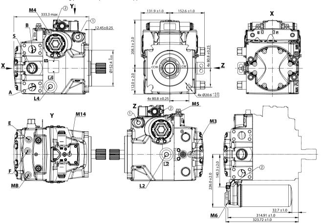
**A/B** system ports: Ø31.5 mm; M12 x 1.75; 20 min. full thread depth **MA/MB** (system), **M3, M6** (charge) gauge ports per ISO 11926-1:  $\frac{9}{16}$ –18 **M4, M5** (servo), **M14** (case) gauge ports per ISO 11926-1:  $\frac{7}{16}$ –20 **L2, L4** – Case drain ports per ISO 11926-1:  $\frac{15}{16}$ –12
