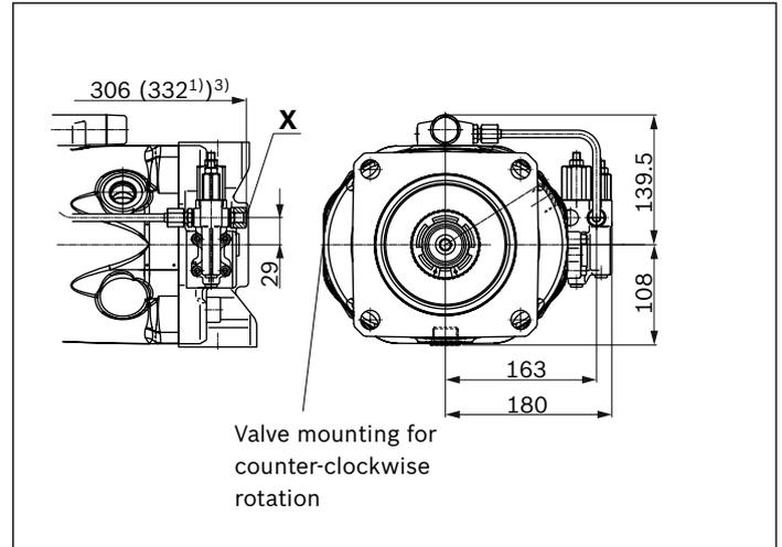
▼ **DRG – Pressure controller, remotely controlled; mounting flange D**
