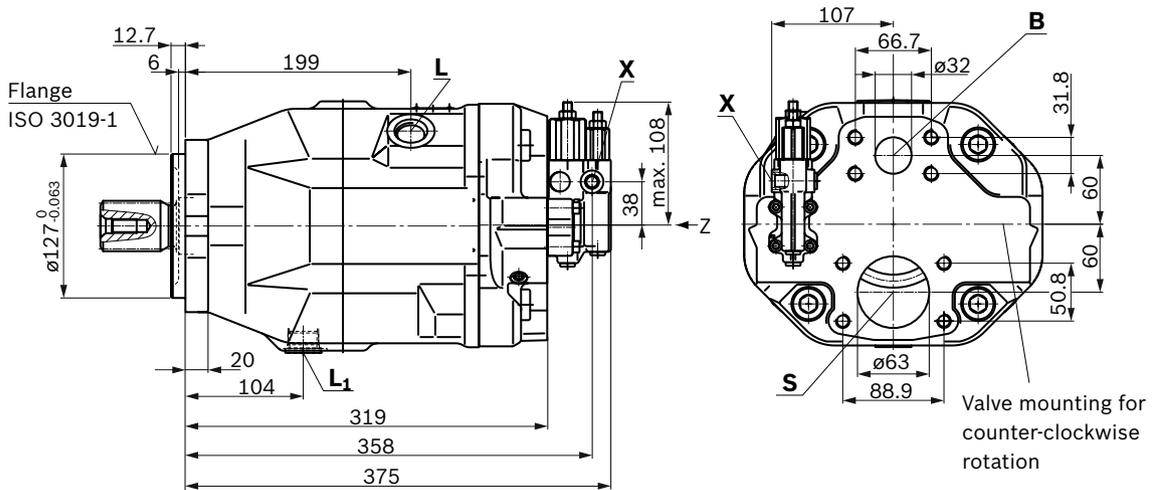
**DRF, DRS, DRSC – Pressure and flow control, port plate 11 and 12; mounting flange D (SAE-D; 152-4)**
