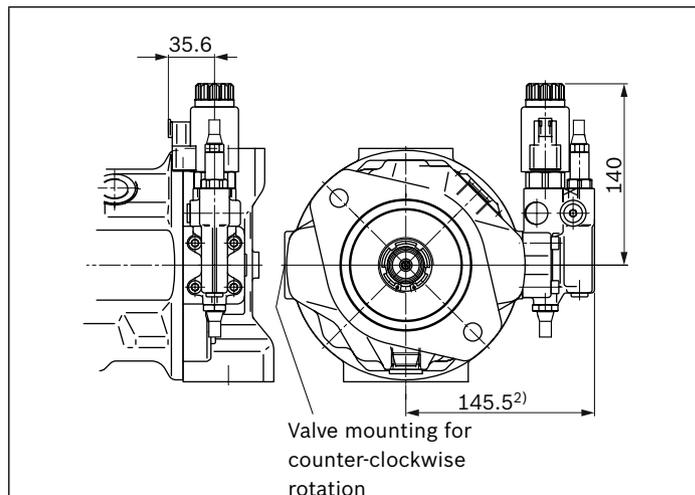
1) ER7. 180.5 mm if using an intermediate plate pressure controller
