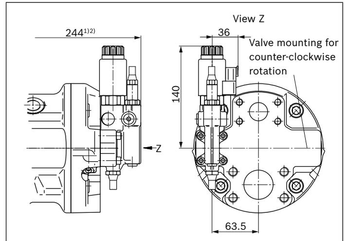
1) ER7. 279 mm if using an intermediate plate pressure controller
