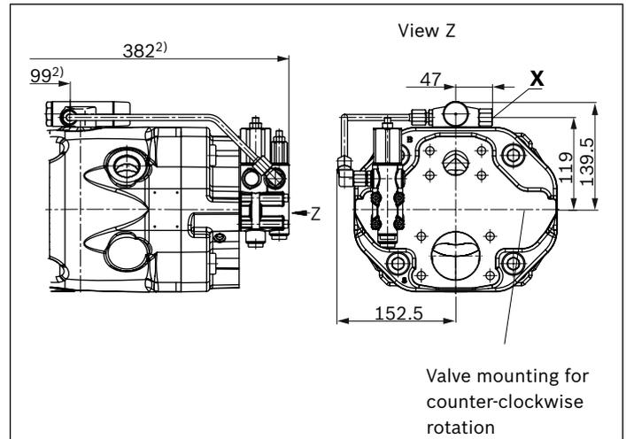
▼ **DRG – Pressure controller, remotely controlled**
