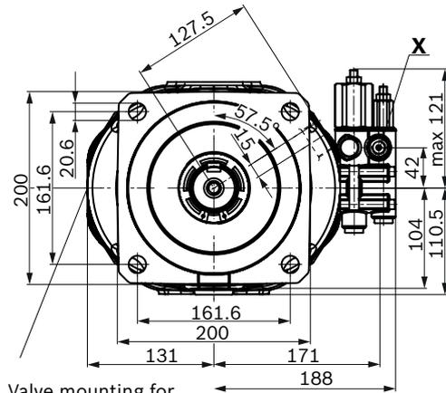
Valve mounting for counter-clockwise rotation
