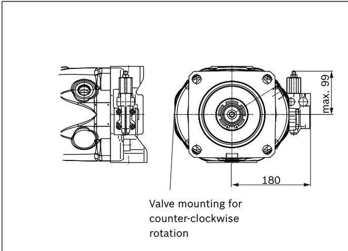
▼ **LA.DS – Pressure, flow and power controller; mounting flange D**
