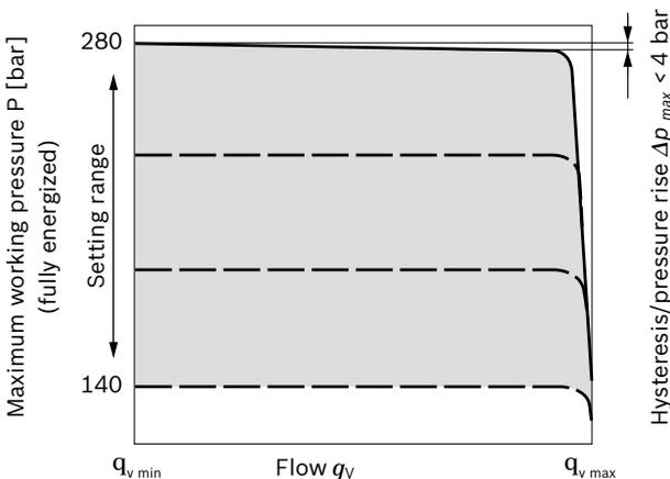
Characteristic curves valid at  $n_1 = 1500$  rpm and  $\theta_{\text{fluid}} = 50$  °C.
