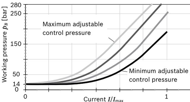
Hysteresis static current-pressure characteristic curve < 3 bar.
