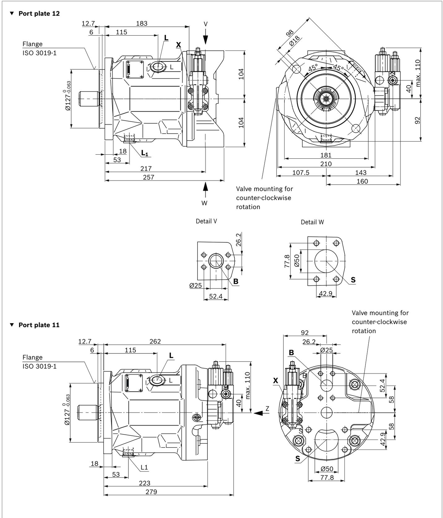
**DRF, DRS, DRSC – Pressure and flow control, port plate 12; mounting flange D (SAE-C; 127-4) and U (SAE-D; 152-4)**
