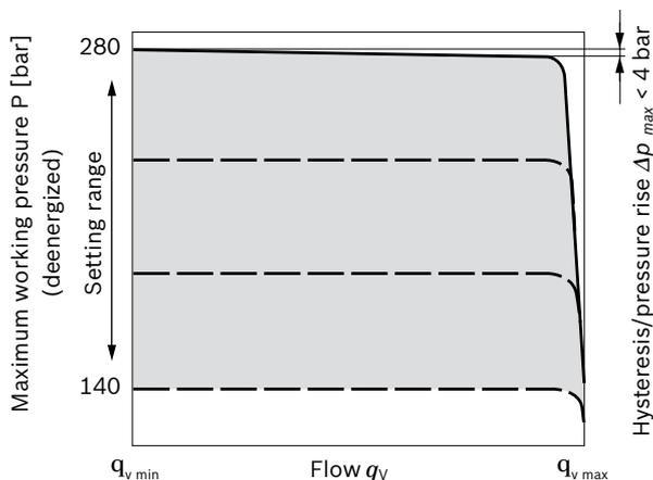
Characteristic curves valid at  $n_1 = 1500\ rpm$  and  $\theta_{fluid} = 50\ ^\circ C$ .
