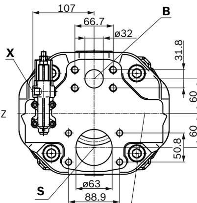
Valve mounting for counter-clockwise rotation
