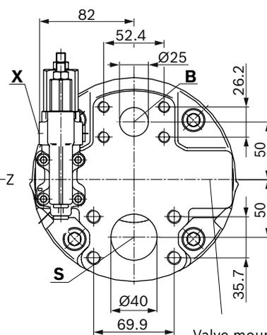
**DRF, DRS, DRSC – Pressure and flow control, port plate 11 and 12; mounting flange D (SAE-C; 127-4)**
