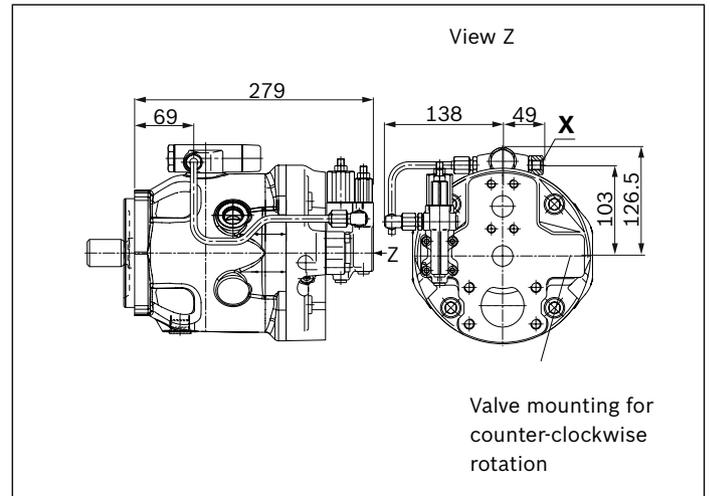
▼ **DRG – Pressure controller, remotely controlled**
