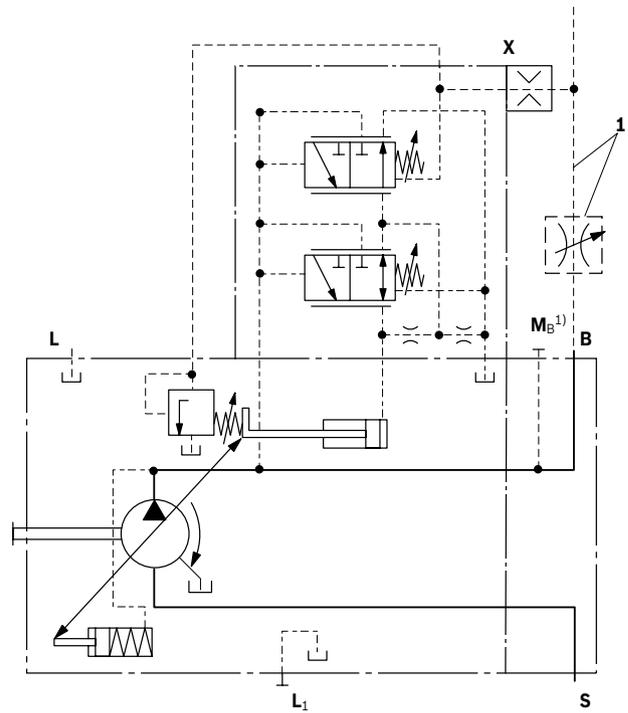
▼ **Circuit diagram LA.S** with separate flow control
