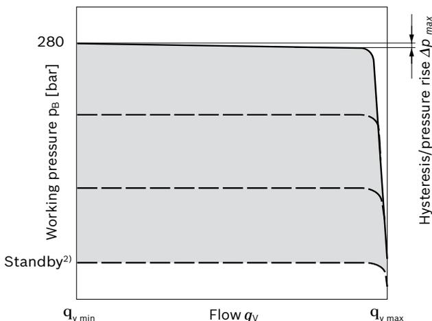
Characteristic curve valid for  $n_1 = 1500$  rpm and  $\theta_{\text{fluid}} = 50$  °C.
