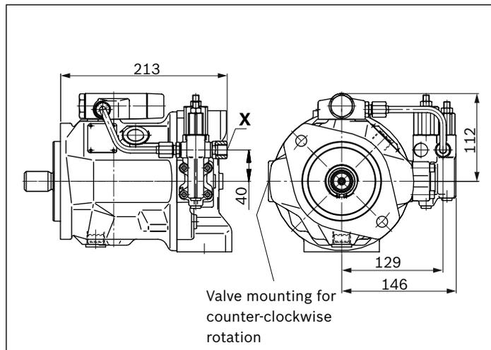
▼ **DRG – Pressure controller, remotely controlled**
