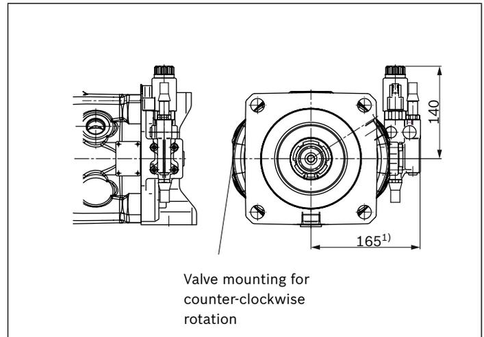
1) ER7. 200 mm if using an intermediate plate pressure controller
