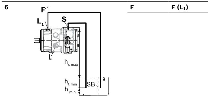
A check valve in the drain line is only permissible in individual cases. Consult us for approval.
