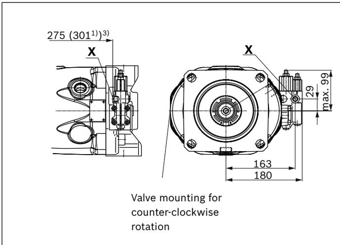
▼ **ED7./ER7. – Pressure controller, electric; mounting flange D**
