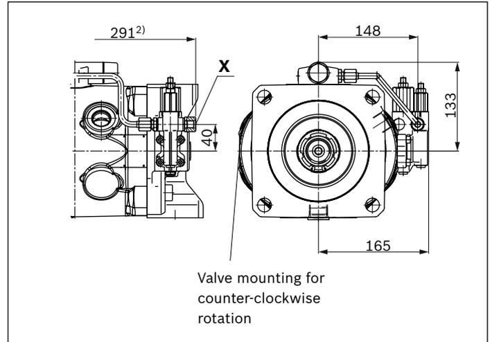
▼ **DRG – Pressure controller, remotely controlled**
