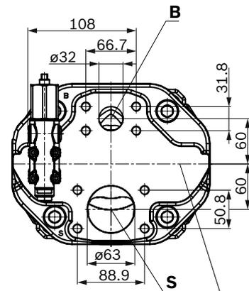
Valve mounting for counter-clockwise rotation
