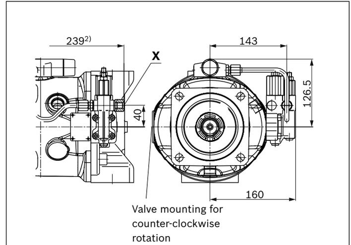
▼ **DRG – Pressure controller, remotely controlled**
